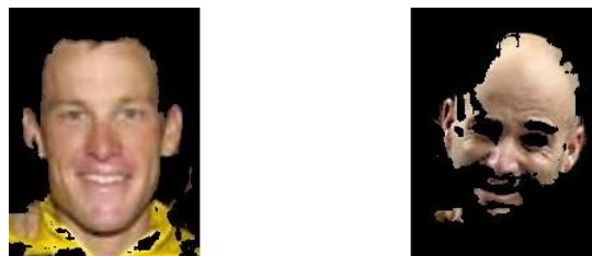
Figure 3.6: Example images of a good skin detection compared to a lossy detection
