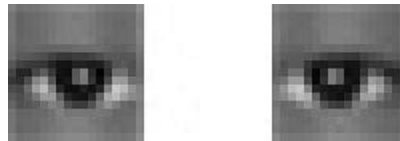
Figure 4.24: Left and right eye template (17x17 pixels)
