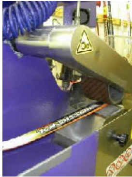
Figure 13: Ski base stone grinding (source www.ultratune.net )
